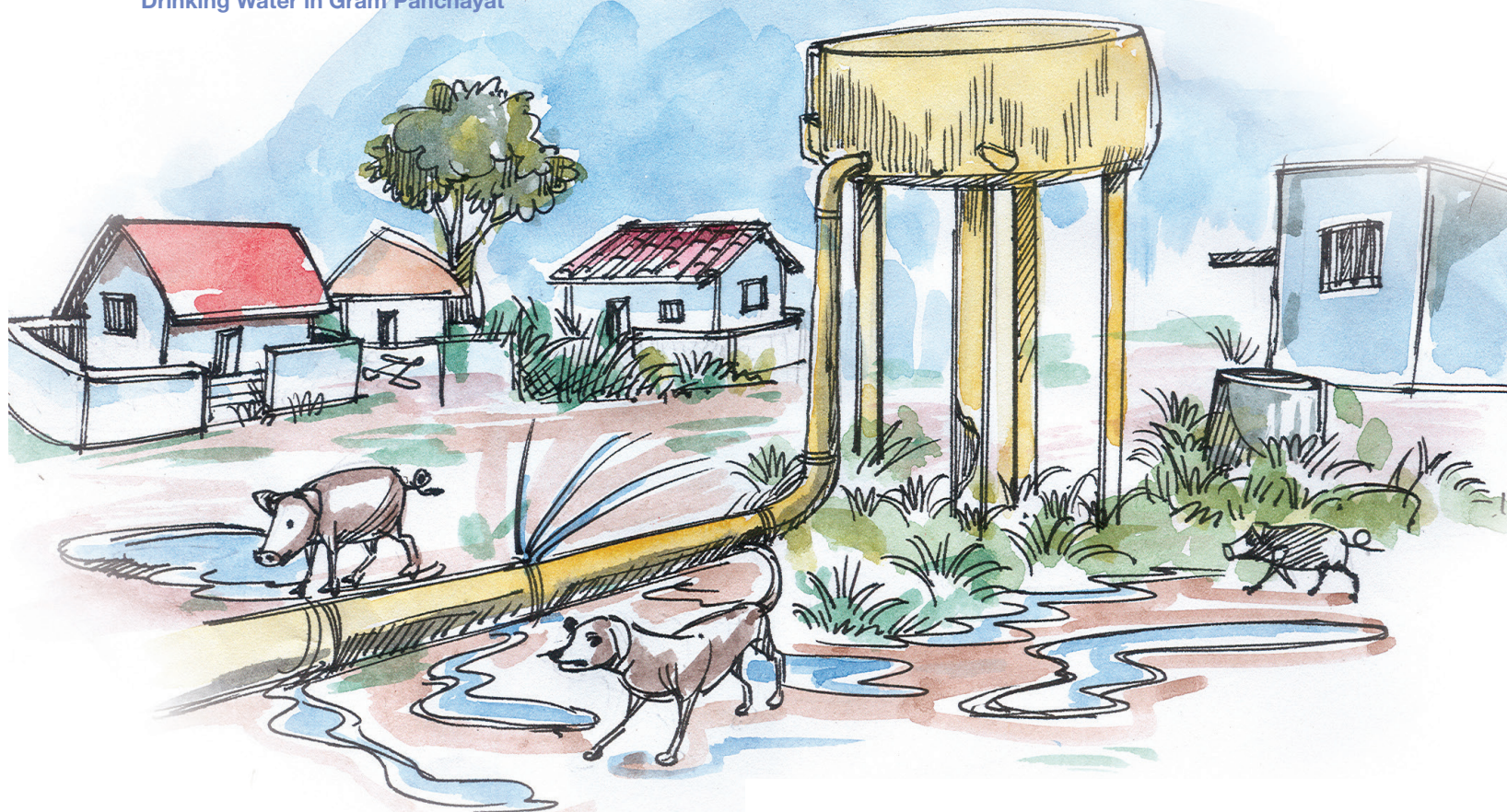
Sanitary risk around a reservoir
